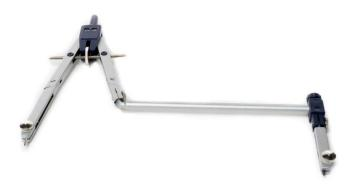
The biggest circle or arc you can make with the extension beam fully extended is 22 inches diameter<sup>2</sup>. The compass is not easy to control of you make the circle that large, but 20 inch diameter is easily managed. That's large enough to put a small goat through.
